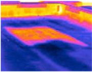
roofs with either a smooth or gravel surface, built-up or single-ply membranes. For smooth-surfaced roofs, a short wave imager will provide more accurate results especially if the roof is painted with a reflective coating. All infrared data should be verified by performing an invasive core sample or moisture meter reading.
